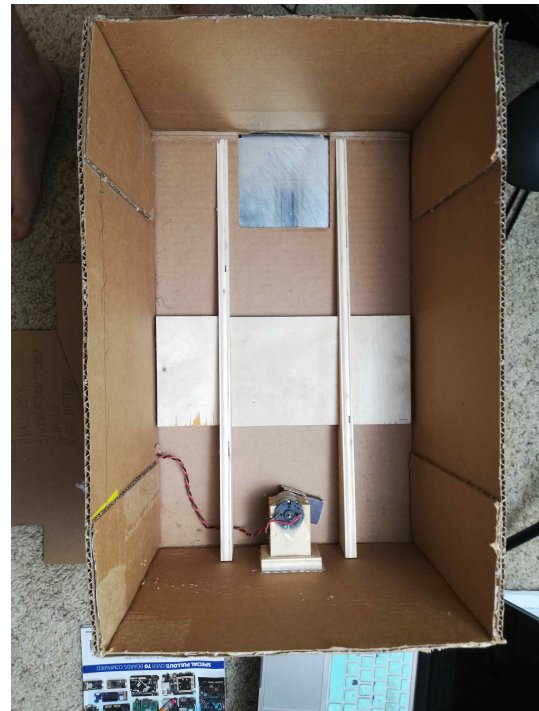
Ping-Pong Ball Hopper With Ramp Removed, Showing Vibration Motor
